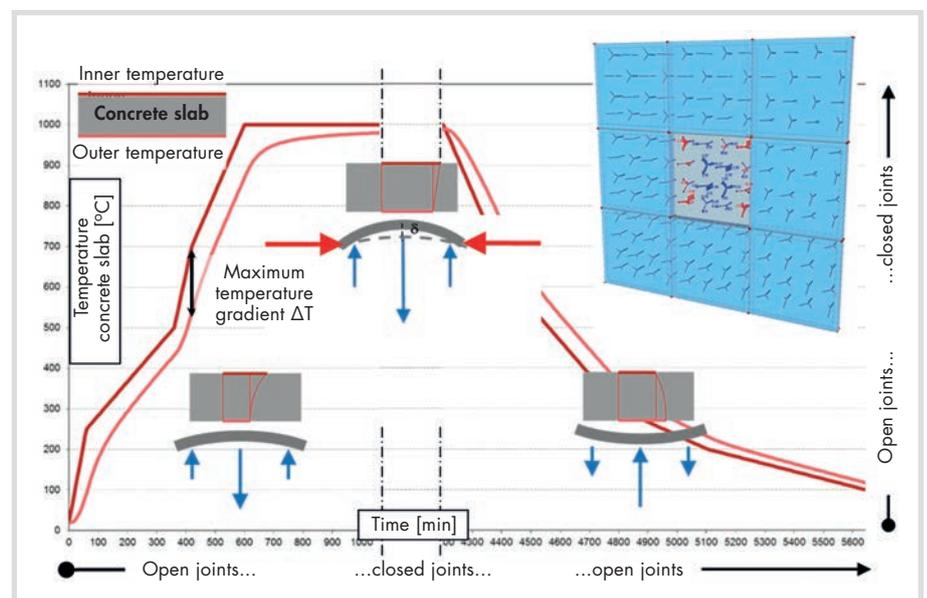
Fig. 10. Furnace cycle of a back-anchored concrete panel.
