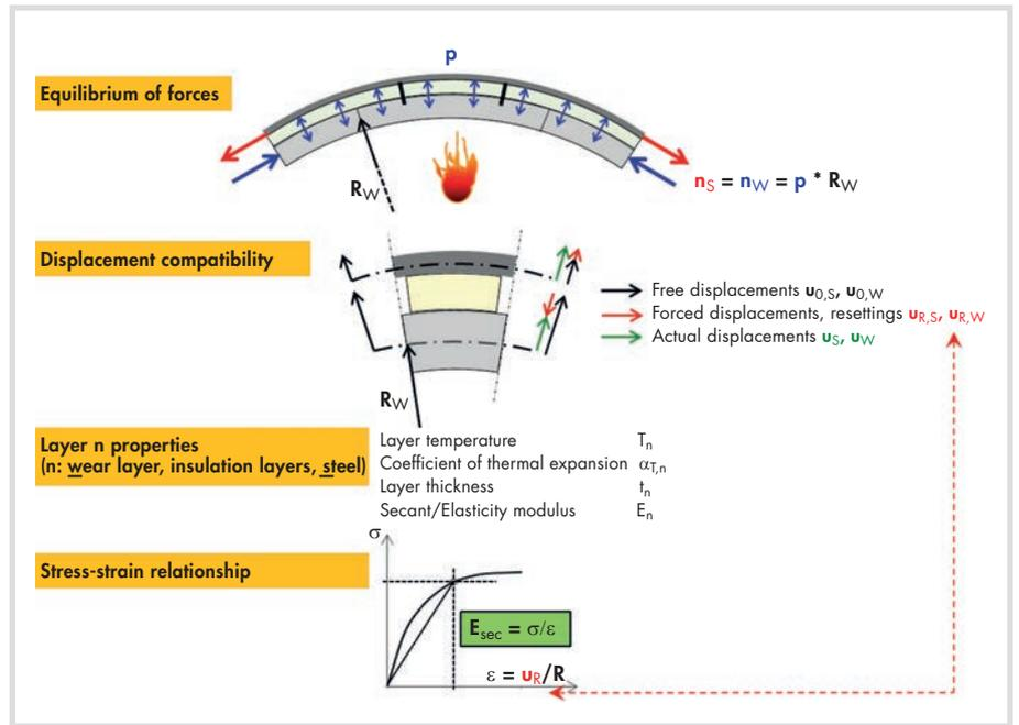
Fig. 2. Mechanical principles for the structural elements' interaction.
