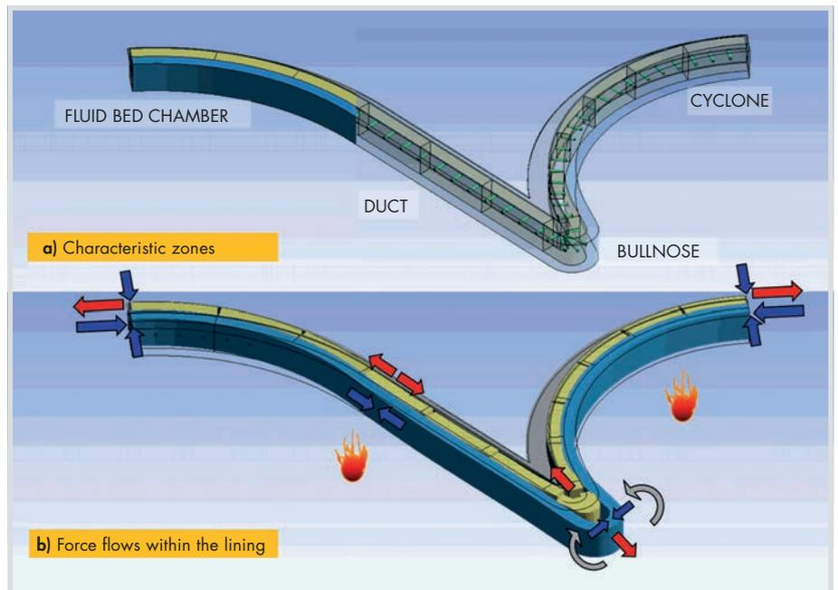
Fig. 3. Different zones result in different behavioural characteristics.
