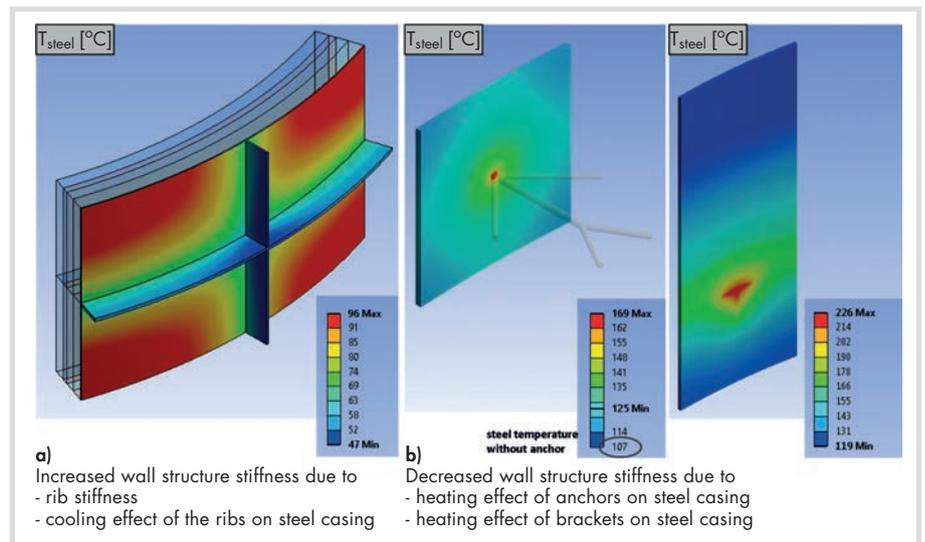
Fig. 4. Changed steel temperatures mean changed stiffness of the entire layer structure.
