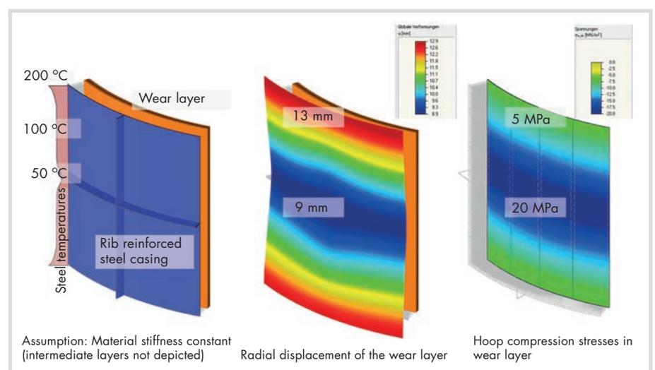
Fig. 5. Influence of the changed system stiffness on the behavioural characteristics.
