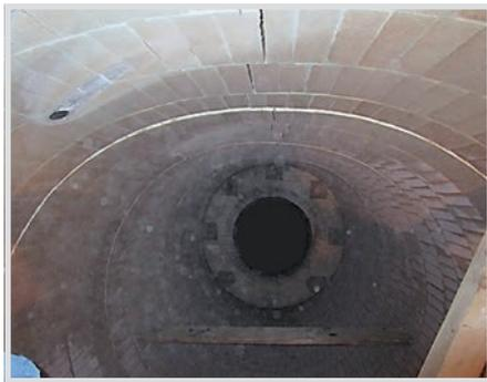
Fig. 8. Result of plasticized material: Lowering of the wear layer in a horizontal cylinder.
