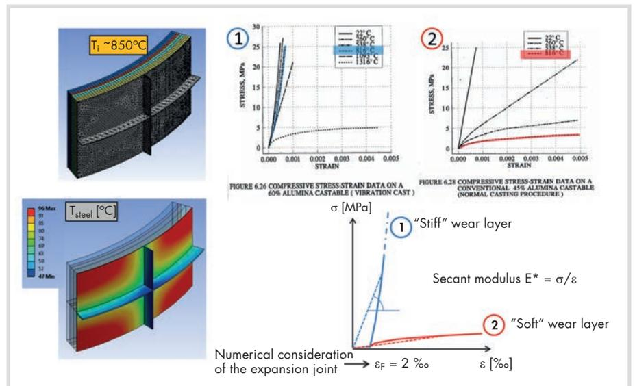
Fig. 6. System and comparison of differently stiff wear layers.
