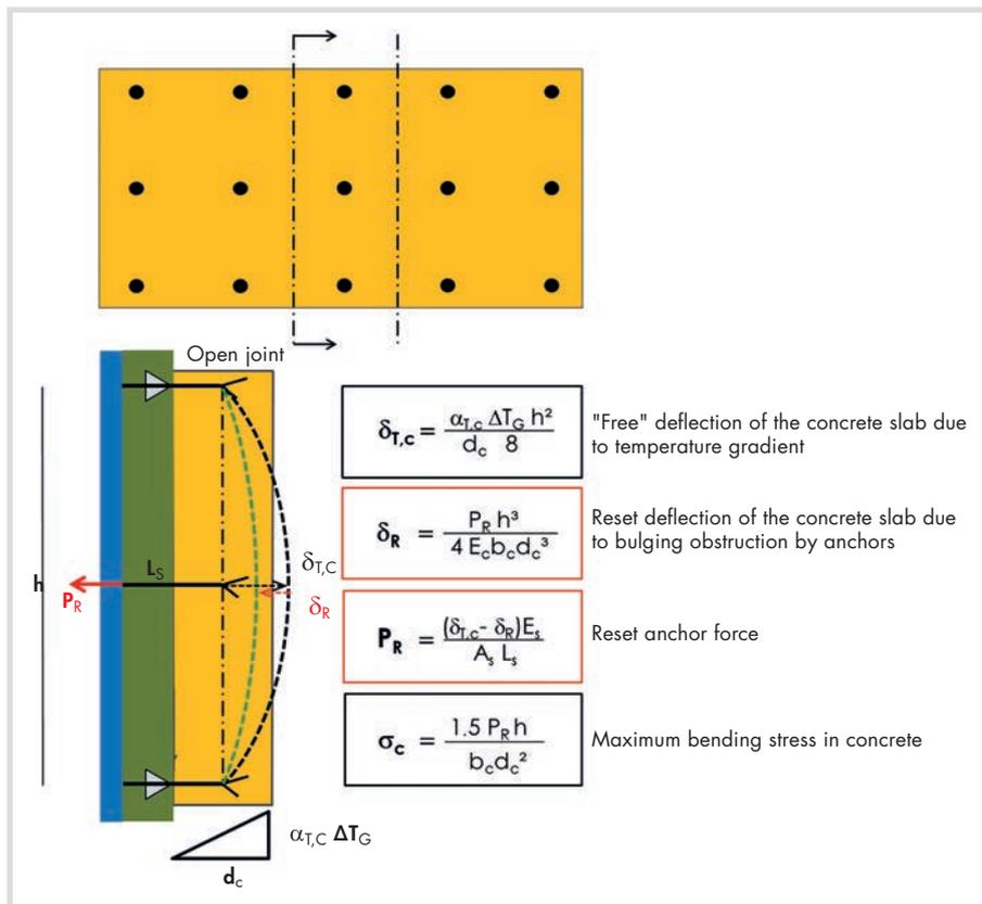
Fig. 11. Computation principle for determining anchor forces and layer stresses.
