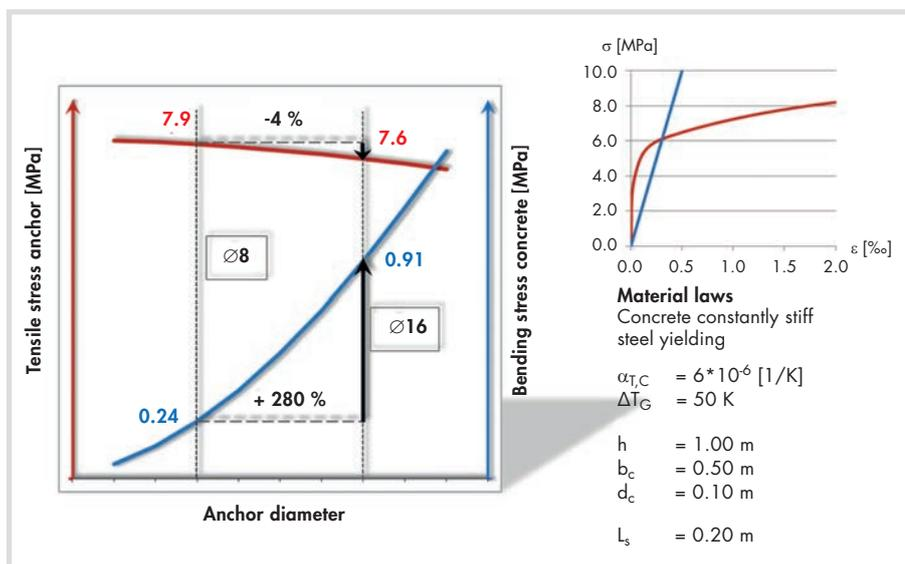
Fig. 12. The use of more powerful anchors does not necessarily bring only advantages!
